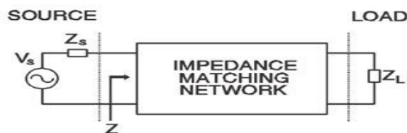
Fig. 6.26 Typical Impedance Matching Network
